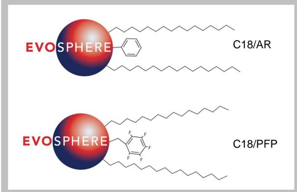
Figure 2 shows how two predominantly C18 phases, both in the USP L1 category, can offer orthogonal selectivity for acids, bases and neutral compounds. This makes these phases highly complementary to each other when developing a new method from scratch. The inclusion of a second ligand in these phases imparts extra mechanisms of interaction such as steric, pi-pi and ion charge.
