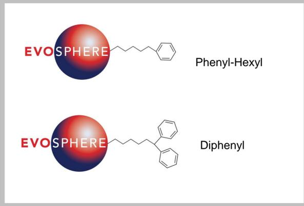
Although the Phenyl phases shown in figure 3 appear similar the addition of the branched structure in the Diphenyl phase chemistry leads to significant selectivity changes due to the extra steric interaction that occurs around the branched structure. With multiple interactions taking place difficult to resolve compounds, such as positional isomers and metabolites, are no longer the problem they once were.
