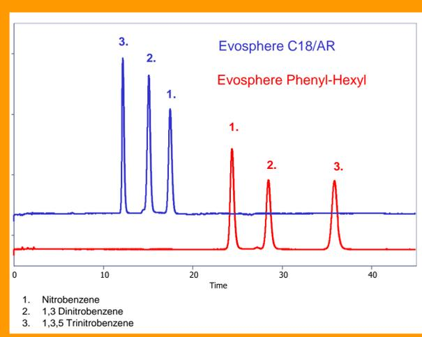
Figure 4 shows how a selection of positional changes on explosives can be separated on two contrasting stationary phases. Both phases are based on monodisperse fully porous particles (MFPP) so provide high efficiency and sensitivity. However it is the choice of stationary phase chemistry which offers the most in terms of resolution and selectivity. The Evosphere C18/AR giving a different elution order to that of a phenyl-hexyl bonded phase.
