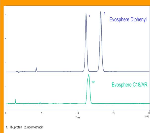
Figure 5 shows how the extra selectivity of the Diphenyl stationary phase offers enhanced resolution compared to an alternative hydrophobic/aromatic containing stationary phase.
